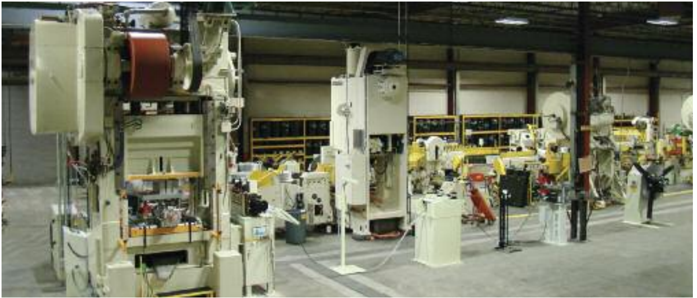
The 70-ft.-long 400-ton press line includes a knurling machine that profiles the strip coming from the feed line. Two loops even out material flow—one loop lies between the decoilers leading to the straightener and out into the knurling tooling and then into the profiling station, and a second loop lies between the profiling station and the press feeder.
